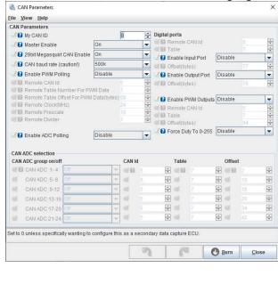
The Megasquirt 2 and Microsquirt requires a different firmware for the gauge. See the product page to download the firmware and program the gauge with it. The gauge will use dash broadcasting instead of requesting the data at the ECU directly.
