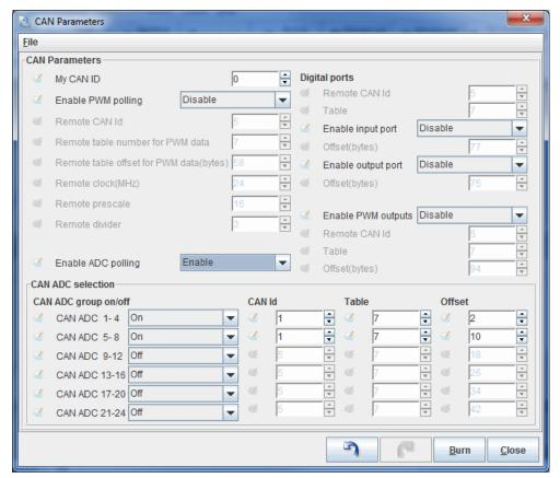
Under the Advanced Engine menu, you can enable thermocouple input under the EGT / Thermocouple Inputs screen. EGT channels 1 through 8 correspond to CAN ADC01 through CAN ADC08, as shown in the screen below. For Calibration, set Temp at 0V to 32 řF or 0 řC, and Temp at 5V to 2282 řF or 1250 řC.
