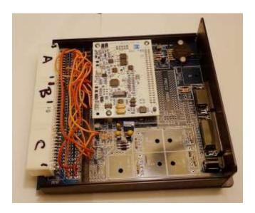
The DIYPNP kits are a product offered by <a href="www.diyautotune.com">www.diyautotune.com</a>. The kit that has the right harness plugs for the Rav4 is the DIYPNP Nippon Denso 76pin Unassembled Kit [DIYPNPN76-K].
